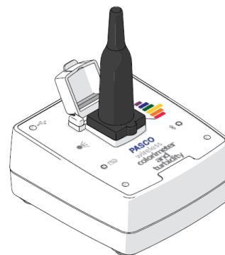
Figure 1. Ampoule cap covering an ezSample Snap Vial ampoule inserted into the test chamber.
