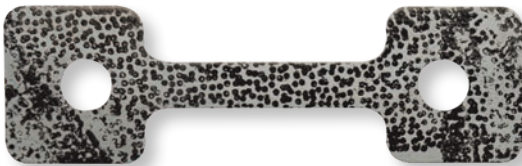
SPECIMEN WITH APPLIED SPECKLED PATTERN
