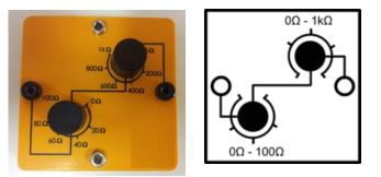
The potentiometer module holds a 0-100- $\Omega$ -potentiometer and a 0-1-k $\Omega$ -potentiometer. Both are serially conneted, so that the potentiometer can attain resistances between 0  $\Omega$  bis 1100  $\Omega$ . The measuring error amounts to 5  $\Omega$  for the small resistor and 20  $\Omega$  at other one. The maximum current amounts to 190 mA.
