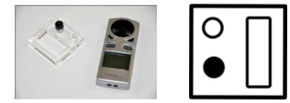
The anemometer can measure the wind speed and displays it in different units. The device can be switch on /off by holding the left button (red circle) for 2 seconds. The unit starts blinking, if the left button is held für 4 seconds. Now, you can change the unit with the right button (plus symbol). The unit can be confirmed by pushing the left button.
