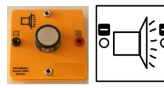
The horn starts making a noise from 0.7 V.
