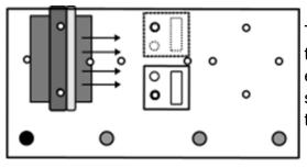
To measure the wind speed you have to remove the wind turbine from the base unit. Afterwards you plug in the holder for the wind measurement device as you can see in the sketch. For a more precise measurement you can calculate the average from the left and the right measuring point.
