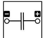
The capacitor module has a maximum capacity of 220 mF and a maximum voltage of 2.5 V. It is protected automatically against an overvoltage.
