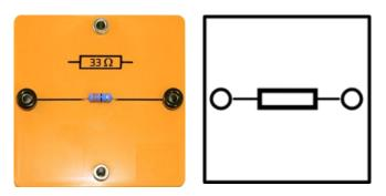
The resistor module contains an ohmic resistor of 33  $\Omega$  with a derivation of 5 %. The maximum power dissipation can amounts to 2W.
