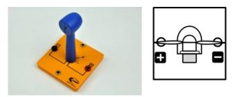
At first the blue wind turbine has to be plugged into the module. The rotor has to be racked at the generator shaft to get a model of a wind turbine. The rotor must not touch the casing to avoid friction, which would considerably impede its rotation. The generator produces a direct current, with its polarity marked on the module. Additionally an angle scale is printed on the module, so it is possible to adjust a certain wind angle.
