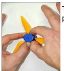
To replace the blades, a small nose is located at head of the hub. If the nose is pressed lightly on a hard surface, the hub-cap can be removed easily.
