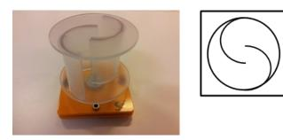
The Savonius rotor module is a model of a wind turbine with vertical rotation axis. The start-up speed amounts to 2 m/s. The open circuit voltage amounts to 0.4 V when there is a wind speed of 5 m/s.
