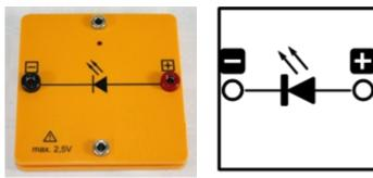
Inside the LED-module, there is a red LED with a wavelength emission of 697 nm. There has to be a minimum voltage of 1.7 V to light up the LED.
