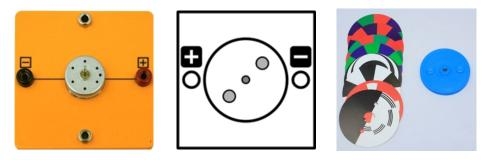
The motor module contains a DC-motor, which rotates in a certain direction depending on the applied voltage. It needs a minimal voltage of 0.35 V to rotate. With the blue plastic disc, you are able to connect the color discs with the motor module. Optical illusions, like the additive color mixing, can be illustrated.
