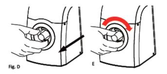
4. While the status light is flashing red, the  $H_2$ -Storage is being filled. Only when the status light flashes green, the cartridge is completely filled. The stick may now be removed by turning it counter clockwise.
